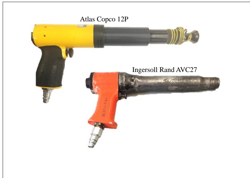
Figure 5.2: Displays the Atlas Copco 12P (top) and the Ingersoll Rand AVC27 (bottom), both of which are tested in the interference-fit bolt experiment. The 12P has a mass of 2.23 \text{ kg} and the AVC27 has a mass of 2.35 \text{ kg} . The weight of the additional moving components, which include the linear rail block and collar is 0.50 \text{ kg} . The total tested weight for the 12P is 2.73 \text{ kg} , and 2.85 \text{ kg} for the AVC27.
